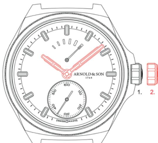
**Note:** Do not forget to push the crown back into position 1 and to screw it down again once you have set the time. This will ensure that your watch remains water-resistant.
